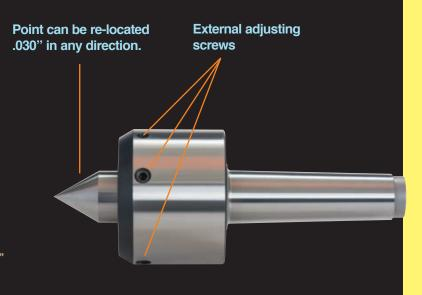
Produced originally as a "customer special", Adjusta-Point live centers have rapidly become a standard catalog item. They are designed specifically for applications when a workpiece's center hole is not quite on center. The adjustable point locates in the center hole, centering the part by offsetting the deviation. The process is similar to indicating a part using a 4-jaw chuck.
