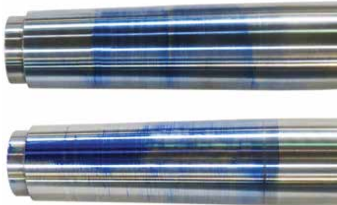
Figure 3. Bluing on a taper gage should be light and even (top). Heavy bluing indicates the taper did not contact the quill interior, while gaps mean the fit was too tight (bottom).
