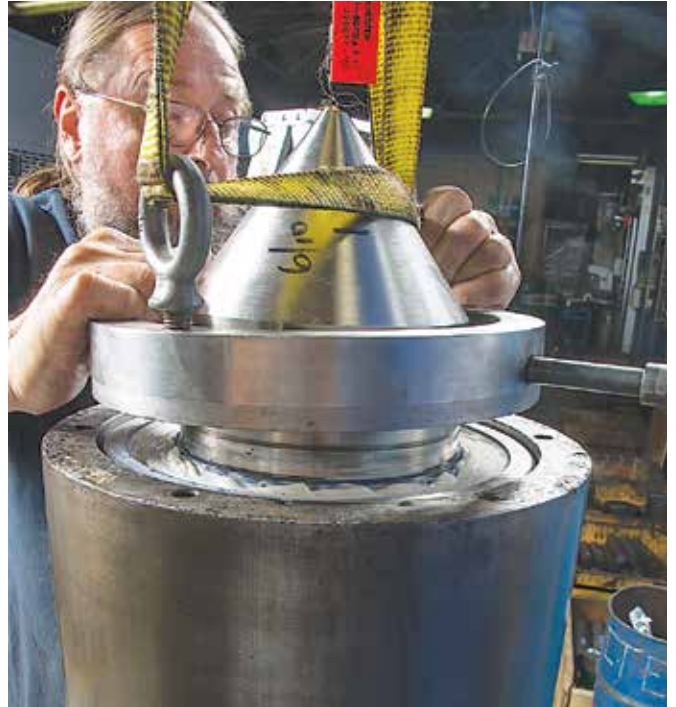
Figure 5. The new spindle is lowered into the repaired quill, achieving a slip fit.
