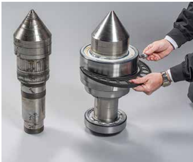
Figure 4a (left). A damaged spindle as received, with failed bearings removed. Figure 4b (right). The remanufactured spindle with new bearings installed.
