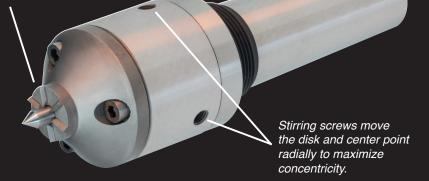
This modified face driver is designed to get a solid grip on small-diameter workpieces. Instead of individual drive pins, the unit features interchangeable drive disks that securely penetrate the face of the part.
