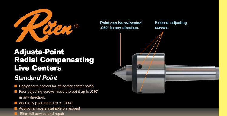
Produced originally as a "customer special", Adjusta-Point live centers have rapidly become a standard catalog item. They are designed specifically for applications when a workpiece's center hole is not quite on center. The adjustable point locates in the center hole, centering the part by offsetting the deviation. The process is similar to indicating a part using a 4-jaw chuck.
