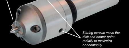
This modified face driver is designed to get a solid grip on small-diameter workpieces. Instead of individual drive pins, the unit features interchangeable drive disks that securely penetrate the face of the part.
